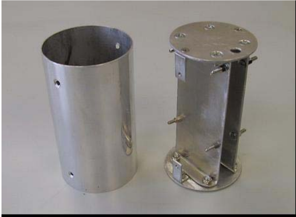
Figure 28: Previous Coke-Can size CanSat [Campbell and others, 2003].
