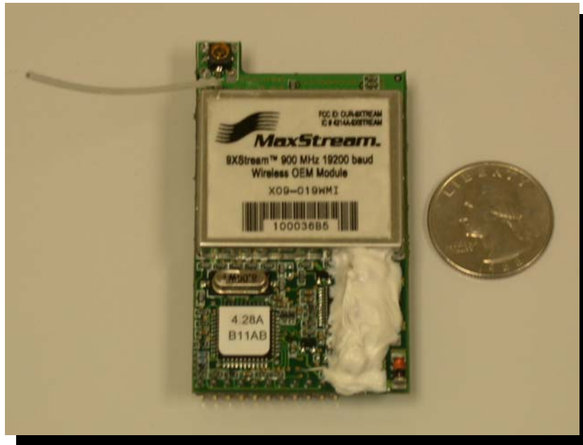
Figure 12: Size of MaxStream XStream™ 900 MHz wireless OEM module.
